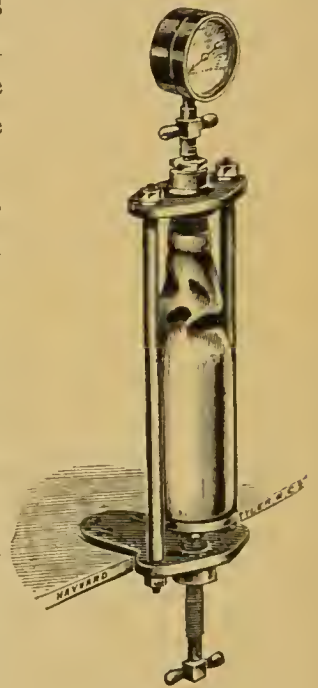
FIG. 112.—Testing Gauge for Codd's Bottles.
